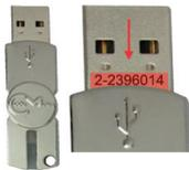
By the way: The serial number of the *CmStick* can be found on the plug-in connector. Now plug the *CmStick* into a free USB port and click the Update button
